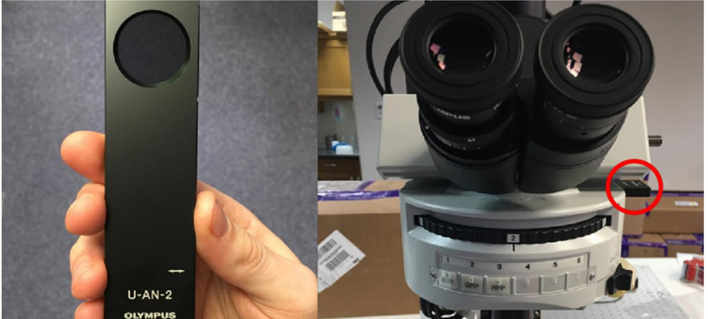
*The image on the left is a U-AN analyser, and the image on the right shows the U-AN analyser inserted into a fluorescent turret on the SliceScope.*
