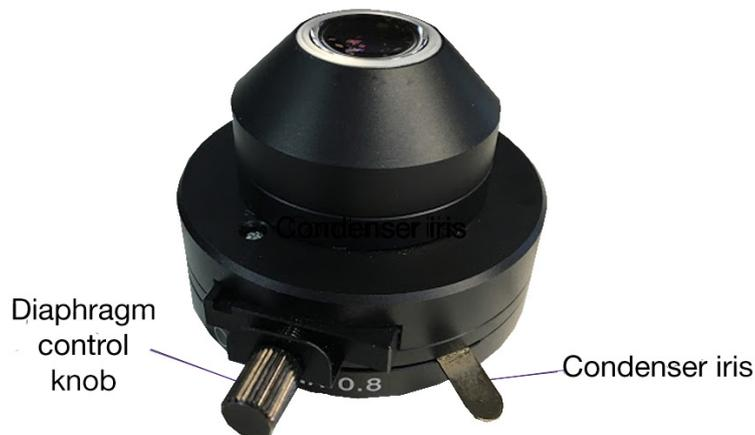
Firstly, pull out the oblique slider and open the oblique iris so the condenser is adjusted for brightfield illumination.
