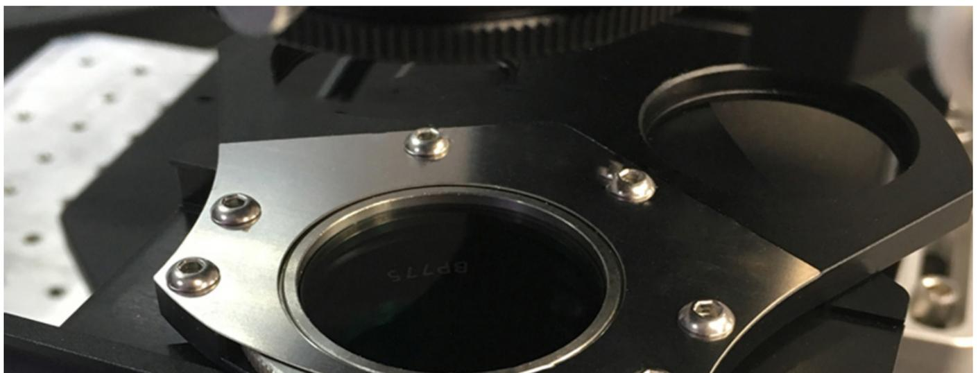
*Filter wheel with rotatable mount, showing the installed polariser*
