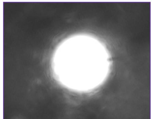
5) Once the condenser has been focused and centred in this way, the diaphragm can be opened so that it is just outside the field of view.
